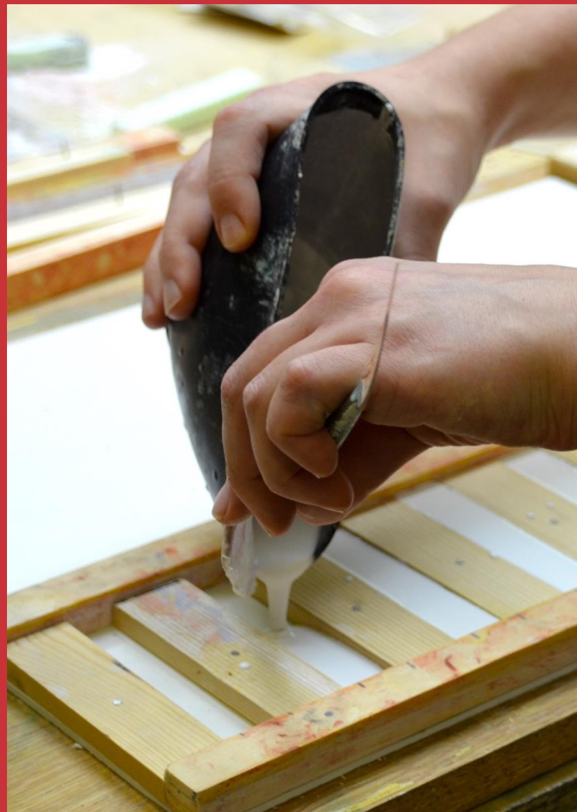
Prikaz vlivanja mešanice izbranega materiala v lesen kalup. Demonstration of pouring the mixture into the wooden mould.
