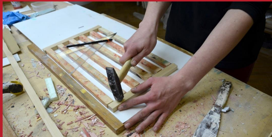
Izdelovanje lesenega kalupa za vlivanje mase. / The process of making wooden mould for the cast.
